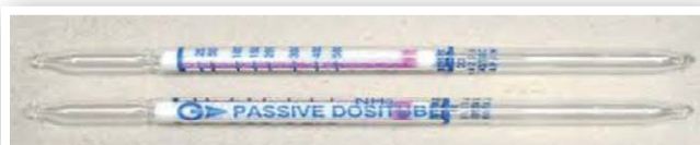
Figure 1: Experimental set-up for measuring ammonia volatilization, August 2022. The dosimeter tube (see below) is placed under the recycling box about 10 inches above the soil surface after N application. It measures exposure to ammonia in parts per million. Note: At this site, the soil was pre-wetted to maximize potential volatilization. Ammonia exposure was measured for five days after nitrogen application.
