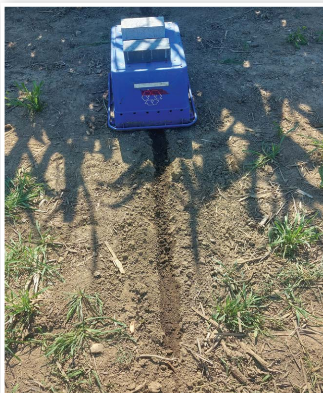
Figure 1: Experimental set-up for measuring ammonia volatilization, August 2022. The dosimeter tube (see below) is placed under the recycling box about 10 inches above the soil surface after N application. It measures exposure to ammonia in parts per million. Note: At this site, the soil was pre-wetted to maximize potential volatilization. Ammonia exposure was measured for five days after nitrogen application.
